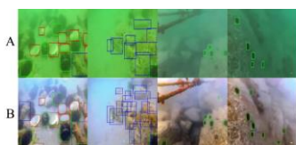
Figure 7: Underwater target detection results before and after enhancement. (A) Real-world underwater images and (B) output of our model for the real-world image. Red boxes represent scallops, blue boxes represent sea cucumbers, and green boxes represent sea urchins.
