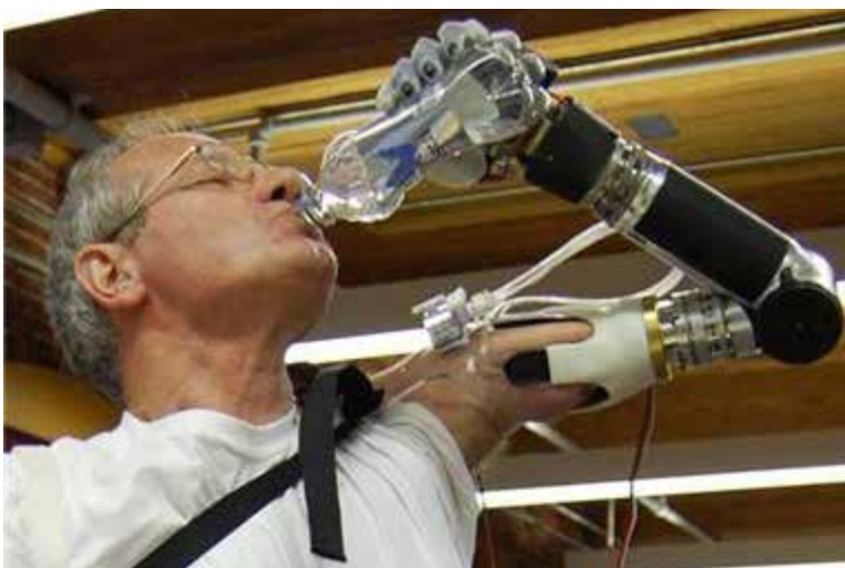
A man drinks water with his Luke arm. The biggest advantage of this prosthetic arm is that it does not require a special mechanism such as buttons; it can be controlled just like a real arm. © Medgadget
