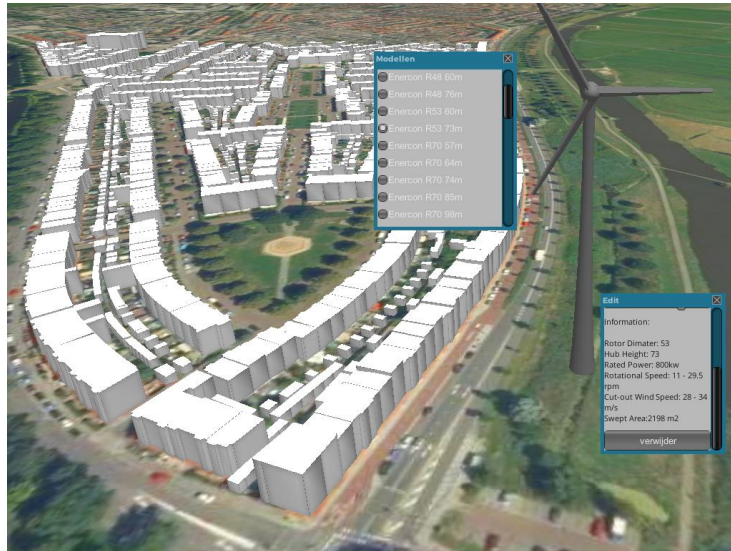
Figure 7. Wind turbine scenario design in Falcon. Users can select different wind turbine types and bring them into the scene as game objects. By placing a wind turbine in the scene, its geometric and technical characteristics are retrieved from the database and are presented.
