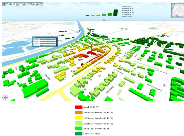
Figure 9. Wind turbine noise impact calculation in Falcon. The wind turbine noise impact is presented real-time both visually (colorized buildings and chart) and numerically (top).
