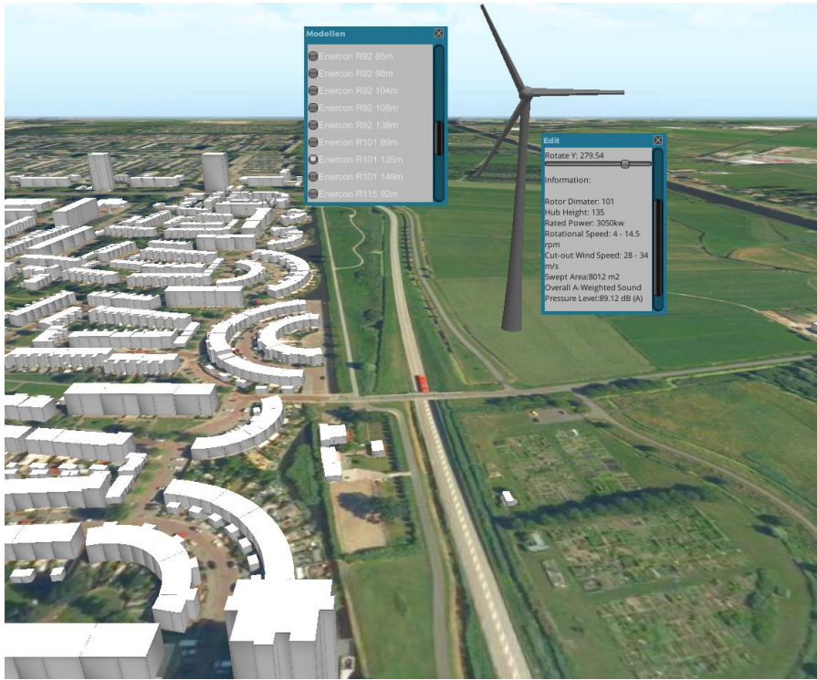
Figure 7. Falcon 3D design platform; designers can add different types of wind turbines into the scene. Once a specific wind turbine is added, its technical information will be queried for further analysis. This information can also be observed by clicking the wind turbine.
