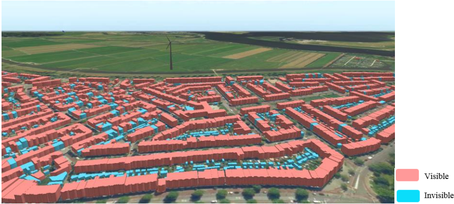
Figure 12. Visibility analysis performed in Falcon. The wind turbine is visible from taller buildings whose line of sight is not blocked by other buildings (pink) while not visible from lower buildings hidden behind taller buildings (blue).
